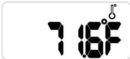
To select the unit of measure for temperature, hold the ON button down for five seconds.
