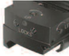
Loosen the two LOCK screws counter clockwise 1/2 turn each using the provided screwdriver. Turn the slotted “UP or LEFT” screws with the provided adjusting disc and screwdriver. The windage adjustment mechanism has limit stops at both ends.
