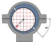
First, try the "0" inserts and see where the point of impact is. In this example, point of impact is 10" high and right measured directly from the center of the target to the center of the three shot group.
